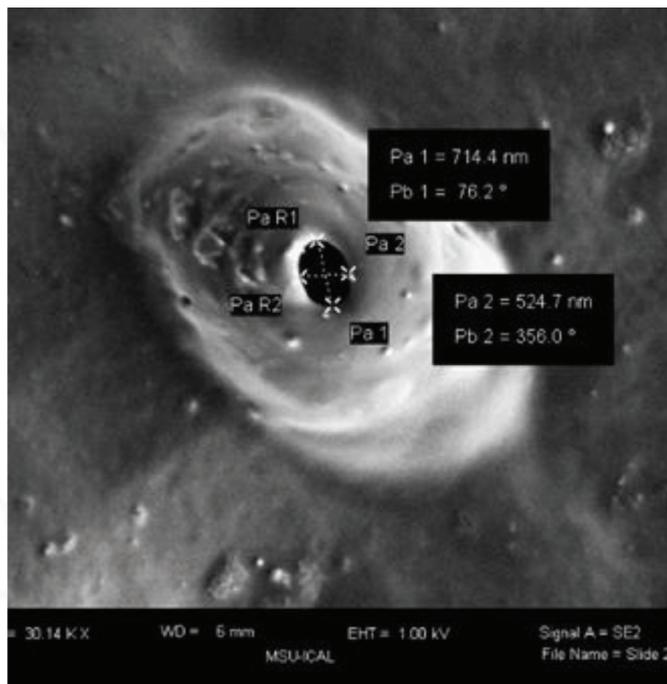
Figure 1. A SEM image of a sub-micron ablation (2 J/cm<sup>2</sup>, 10 shots) on the surface of a compact disc, chosen as a substrate due to its uniform flatness and organic composition. Although slightly ellipsoid, the ablation is clean with no discernible damage corona. This is vital if small structures such as biological cells are interrogated by laser ablation as peripheral damage can cause structural changes in the yet-to-be-analyzed parts of the cell.
