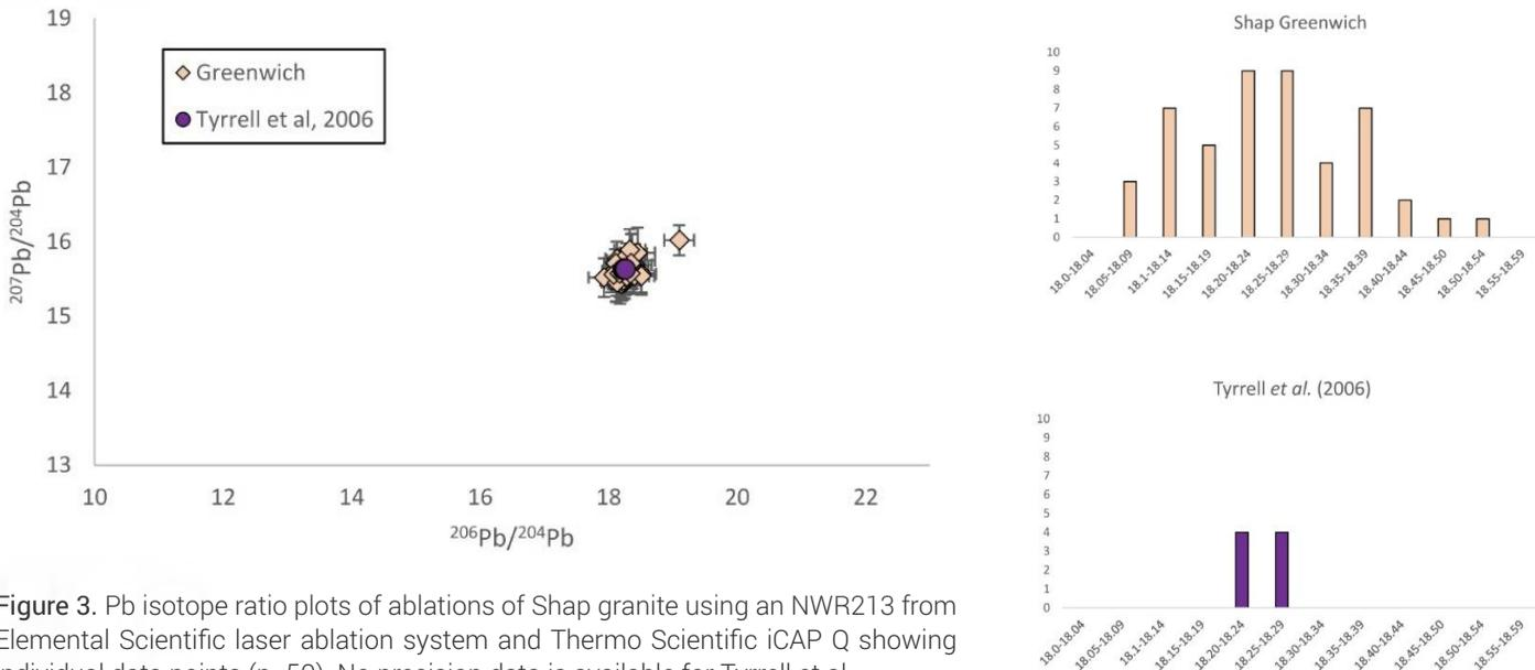
Figure 3. Pb isotope ratio plots of ablations of Shap granite using an NWR213 from Elemental Scientific laser ablation system and Thermo Scientific iCAP Q showing individual data points (n=50). No precision data is available for Tyrrell et al.
