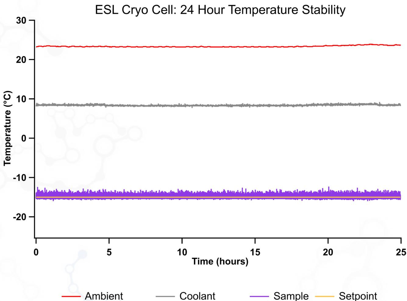
Figure 3. CryoCell stability over a 24 hour period; set point = -15 °C, average temperature at the sample = -15.001 °C with a 2.3 %RSD.
