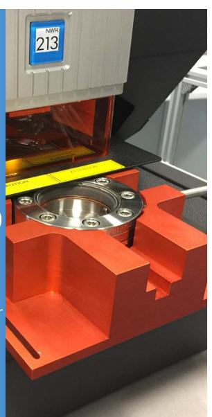
Ultra high vacuum laser ablation chamber with flush window and bolts for safe operation
