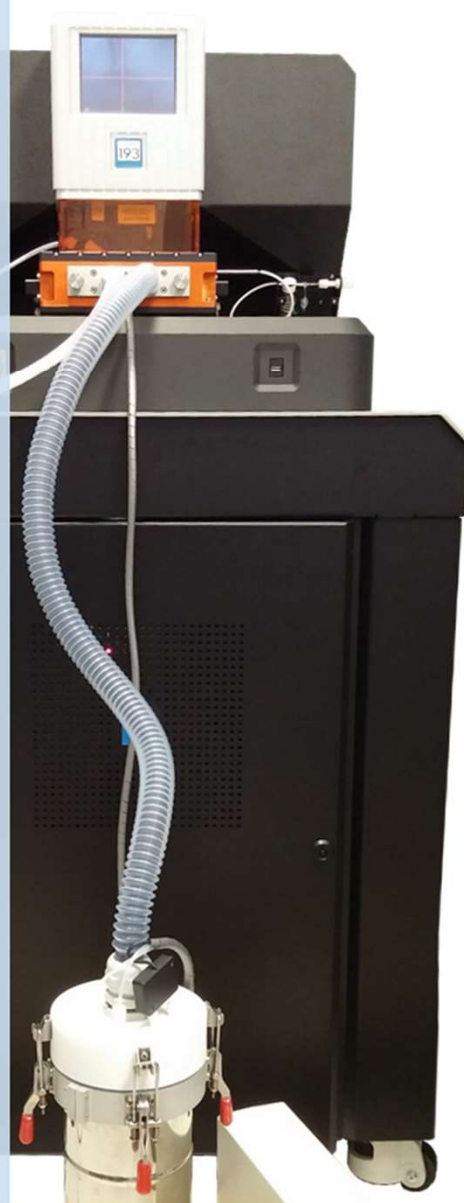
Liquid N 2 cryocell for the NWR Platform
