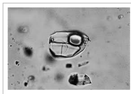
Figure 2. Clean ablation crater, as a result of the rapid, efficient freezing of the CryoCell, on a fluid inclusion in quartz.
